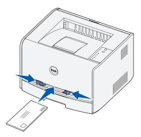
3 Hold both sides of the print media close to the manual feeder and push it into the printer until it automatically engages.
